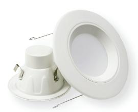
Energetic Lighting's ELDLf series of LED downlight retrofit kits provides an elegant solution for converting existing recessed cans into LED fixtures. Available in 4-inch and 6-inch can sizes operating at 7.5-watt, 11.5-watt, and 18-watt options, with a beam angle of 90°, and dimmable down to 10%. Comprising of a durable die-cast aluminum construction and a LED lifetime rating of at least 35,000 hours, this durable worklight is designed for many years of reliable operation.
